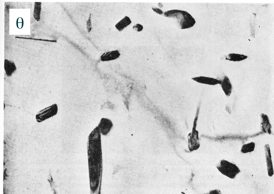
Fig. 5.30 Microstructures at different stages during ageing of Al-Cu alloys. (a) GP zones \times 720\,000 . (b) \theta'' \times 63\,000 . (c) \theta' \times 18\,000 . (d) \theta \times 8\,000 . [(a) After R.B. Nicholson and J. Nutting, Philosophical Magazine 3 (1958) 531. (b) R.B. Nicholson, G. Thomas and J. Nutting, Journal of the Institute of Metals 87 (1958–1959) 431. (c) G.C. Weatherly and R.B. Nicholson, Philosophical Magazine 17 (1968) 813. (d) G.A. Chadwick, Metallography of Phase Transformations , Butterworths, London, 1972, from C. Laird.]
