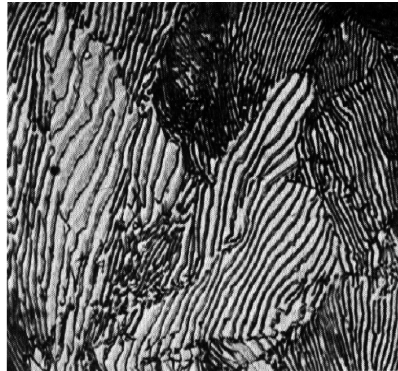
Fig. 5.55 A pearlite colony advancing into an austenite grain. (After L.S. Darken and R.M. Fisher in Decomposition of Austenite by Diffusional Processes , V.F. Zackay and H.I. Aaronson (Eds.), by permission of The Metallurgical Society of AIME.
