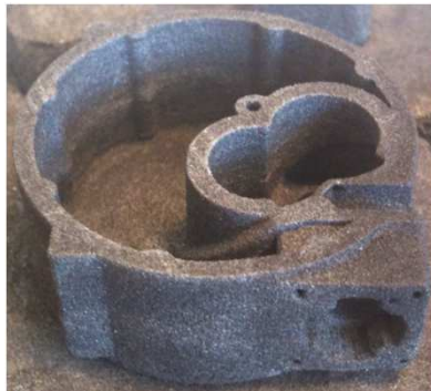
i -AlCuFeB infiltrated by aluminium alloy (98%)
